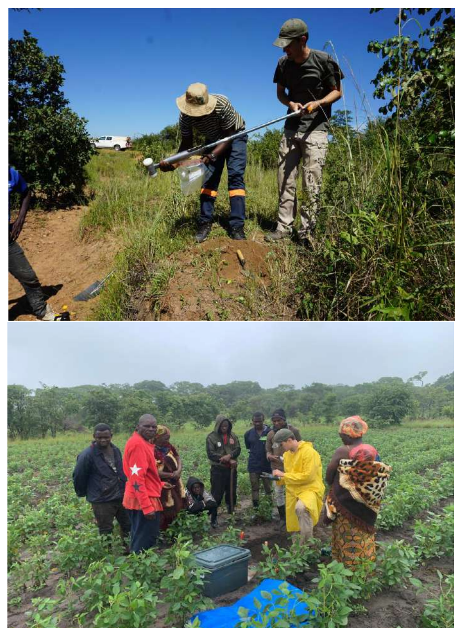
Figure 2: Loose soil sampling for texture and chemical properties. Infiltration measurements using a single ring infiltrometer for field-saturated hydraulic conductivity and undisturbed soil core sampling for bulk density and water retention characteristics.
